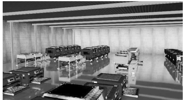
Figure 9: This screenshot from an environment generated by our implementation of the pipeline shows a production area consisting of multiple production lines with AI-generated machines. The lines on the left are identical and have been procedurally composed within step three.
